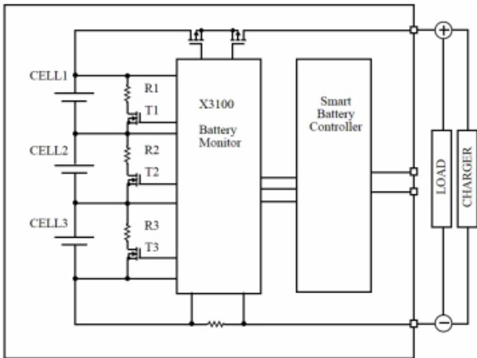
Fig. 3: Cell-Balancing Electronics
