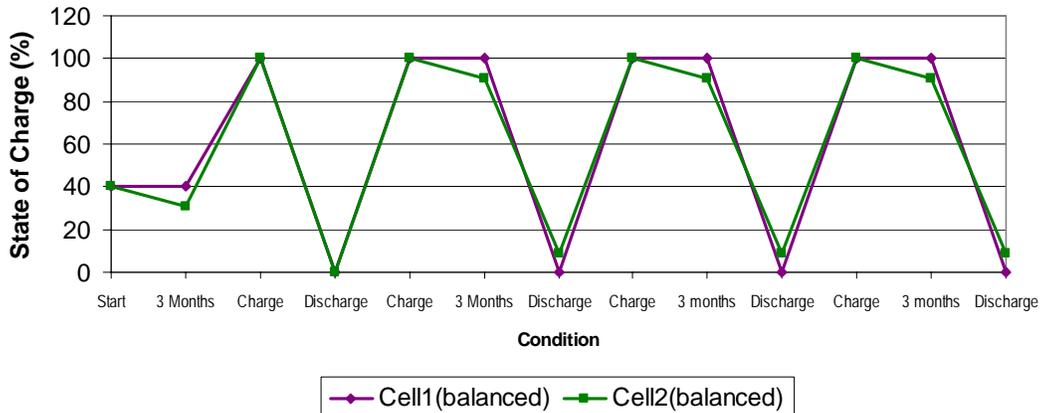
**Fig. 2: Cell Capacity With Cell Balancing**
