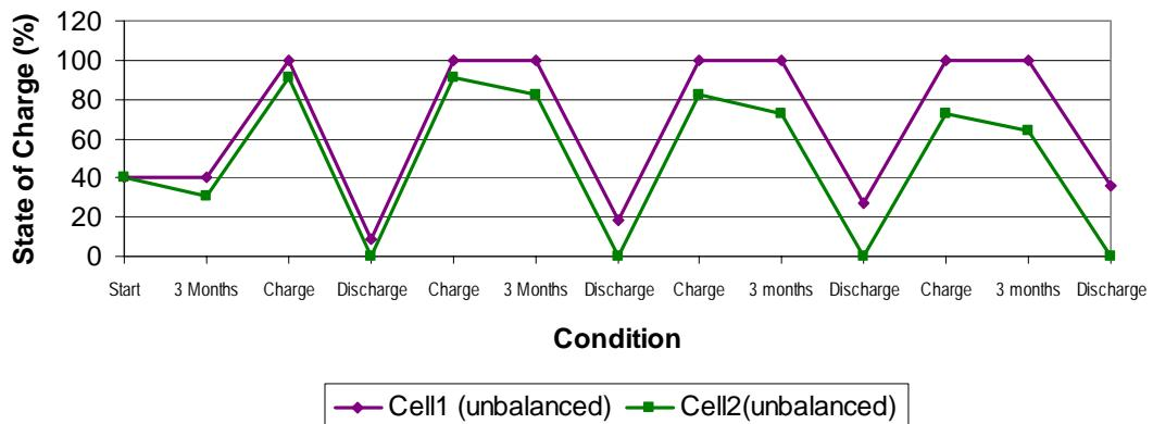
**Fig. 1: Cell Capacity With No Cell Balancing**
