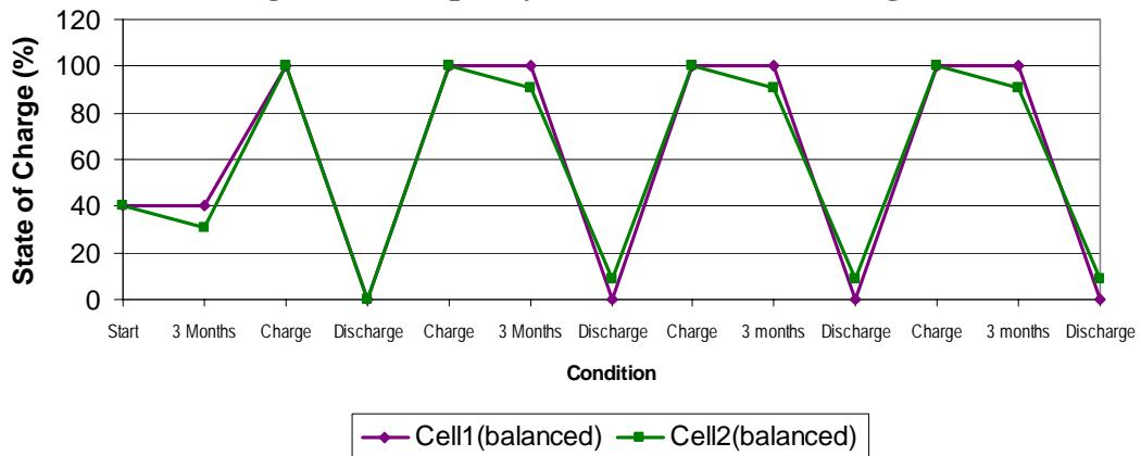
**Fig. 2: Cell Capacity With Cell Balancing**
