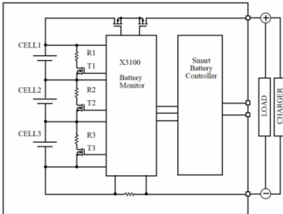
**Fig. 3: Cell-Balancing Electronics**
