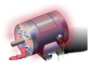
As a rule of thumb, you can generally take a fully loaded Class B insulation motor down to 50 percent speed on constant torque loads without overheating.
