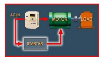
C The ASD can be bypassed in a matter of seconds where other types of speed control may be down for hours or even weeks, while it is being repaired if there is not a spare control.
