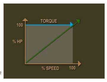
Constant torque loads include most conveyors, positive displacement and reciprocating pumps, and compressors.
