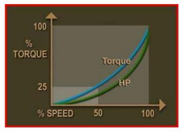
C Variable torque loads include most centrifugal and axial pumps, fans and blowers and many mixers and agitators.
