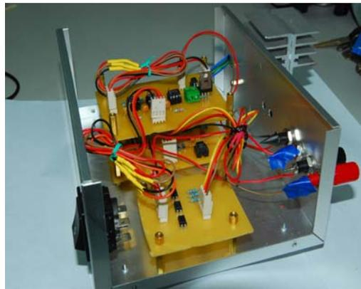
**Fig 7.** The high-pressure GDI injector driving circuit board with last pulse PWM control
