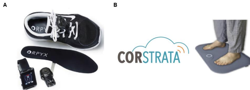
Fig. 3. Wearable devices and sensors. A. SurroSense Rx (Orpyx) smart insoles to screen sustained plantar pressure. Adapted from [12]. B. Corstrata smart thermometric mat – remote temperature monitoring technology. Adapted from [21].
