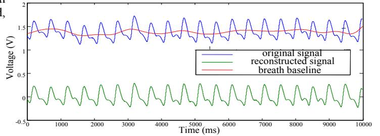
Figure 5. Baseline drift elimination result by WT method
