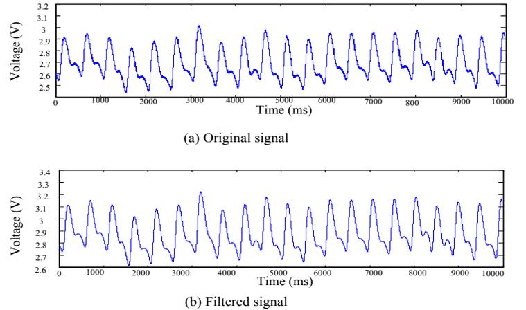
Figure 3. Median filtering and FIR filtering result compared to original signal
