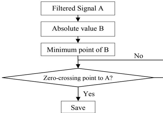
Figure 7. Flow diagrams of the improved differential algorithm
