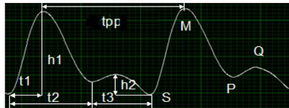
Figure 1. Standard PPG signal and its feature points
